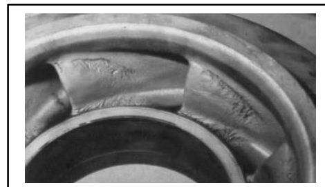
Figure12. Cavitation erosion in a centrifugal pump impeller
